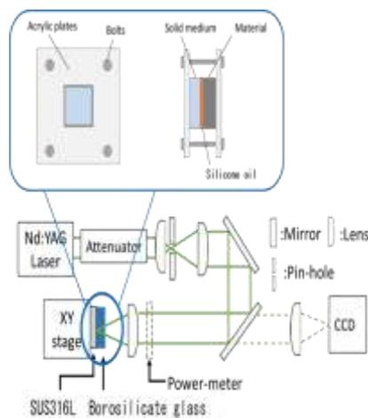
Fig. 5. Silicone oil was poured on the sample surface and pressed firmly with the borosilicate glass
