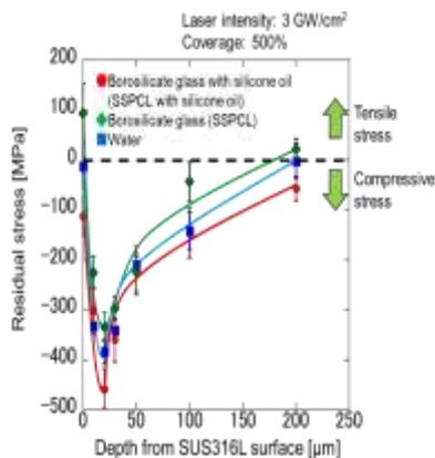
**Fig. 7** Residual stress in laser-peened samples with various plasma confinement layers.
