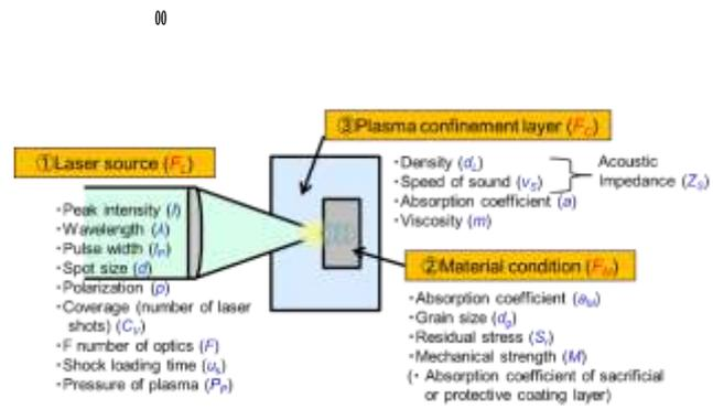
goal is to examine the optimal parameters needed for an efficient laser peening treatment. For this purpose, three factors associated with laser peening are shown in Fig. 1: (1)  $F_L$ , which is related to the laser source, (2)  $F_M$ , which is associated with the material condition, and (3)  $F_C$ , which is related to the plasma confinement layer, have been defined [7-9]. The efficiency of the technique of laser peening can be influenced by controlling these three factors.
