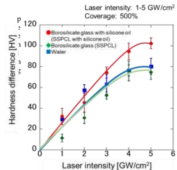
Fig. 6 Surface hardness of laser-peened samples with various plasma confinement layers.
